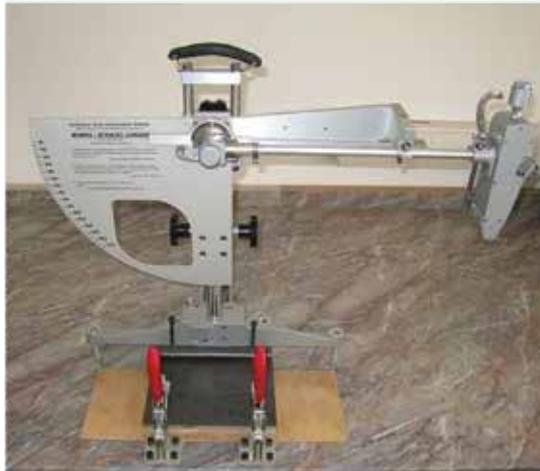
Fig. 1: Portable Skid Resistance Tester SRT 5800
